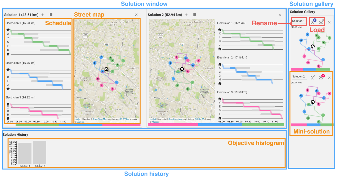
Fig. 3. An overview of the interactive optimisation tool showing its three main components: Solution window, Solution history and Solution gallery (highlighted in blue). Sub-components are highlighted in orange. Interactions are highlighted in red (the rest of interactions in Fig. 4).
