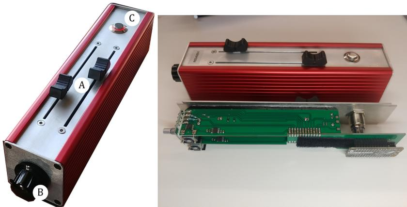
(a) Two actuated sliders (A); Rotary push encoder (B); Push button (C)
