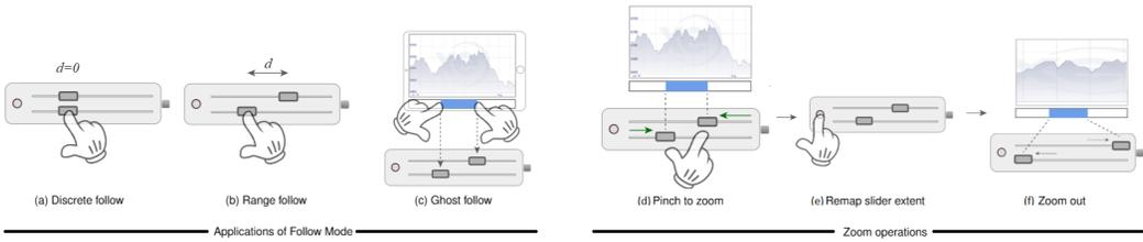
Fig. 2. Filter and zoom using follow mode to pan and joystick mode to expand zoom extent
