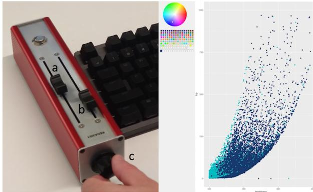
Fig. 4. Choosing colour encoding. Manipulating the colour channel in HSV space: a - left slider: Value; b - right slider: Saturation; c - rotary encoder: Hue.
