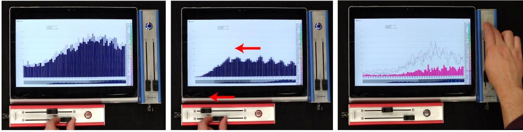
Fig. 5. Use with a 2D chart visualisation with a tablet display: left - range selection (min,max); middle - range sliding to left; right - adding a state to the selection.
