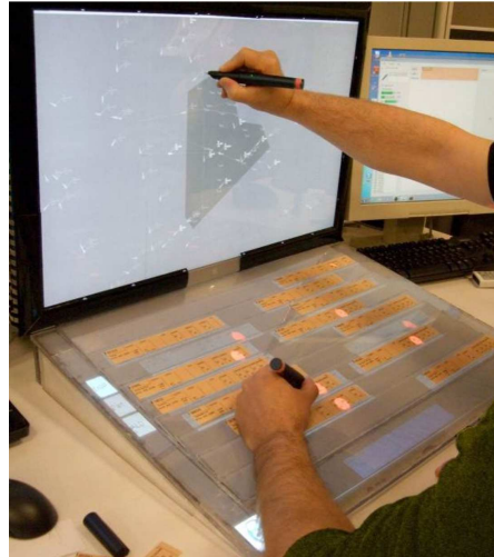
Figure 3: Two controllers using the StripTIC prototype. It features digital pens, augmented radar, stripboard, and paper strips. Image produced from [88]
