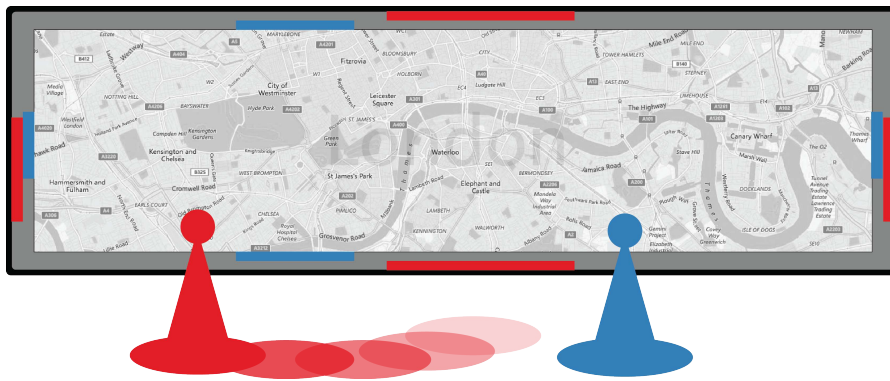
Figure 63: Step Map. The red and blue operators work in front of the wall. Their identity is confirmed by the colored circle around them. The red operator was before directly at the left of the blue one but moved recently more to the left. It is shown by the fading away red circles.
