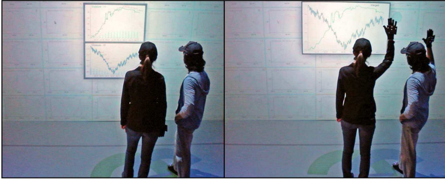
Figure 18: Users doing a visual exploration task on a wall display using hybrid interaction techniques. Here users are doing a merge of two visualizations. It uses proxemics to stack the lenses when the users are close (left) and changes the merge mode to content overlay when they perform a collaborative gesture (right). Image produced from [14]
