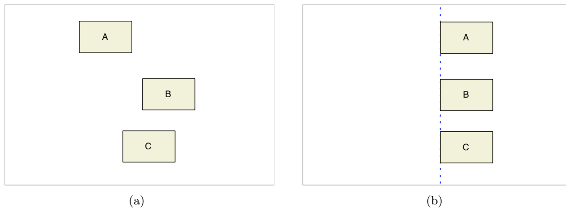
Figure 2.8: Effect on layout due to one-way left-alignment of shapes A and C with shape B. In contrast to Figure 2.6, a guideline is created and all three shapes become aligned with and attached to it.
