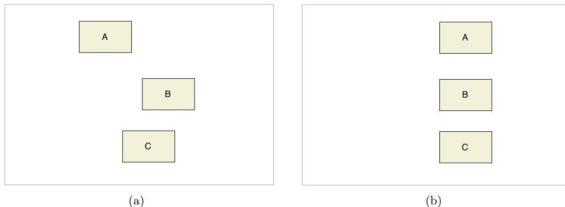
Figure 2.6: Effect on layout due to once-off left-alignment of shapes A and C with shape B. Shapes A and C are moved into line with shape B.
