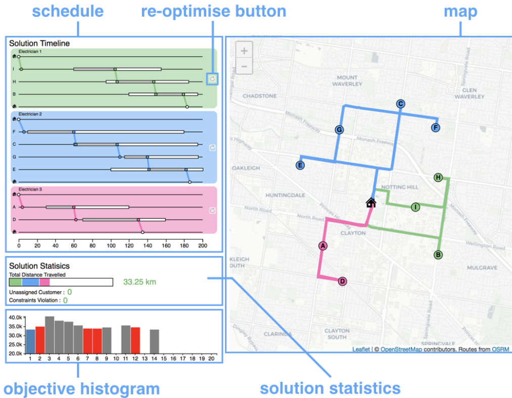
Fig. 4. Study 2 interface. The objective histogram is shown in both SI and MI conditions. The re-optimize button is only available in SI condition. The button turns off (greys out) when it is not possible to improve the solution by reordering the order in which customers are visited by the associated electrician. The button turns on when there is a better solution with a shorter total distance.
