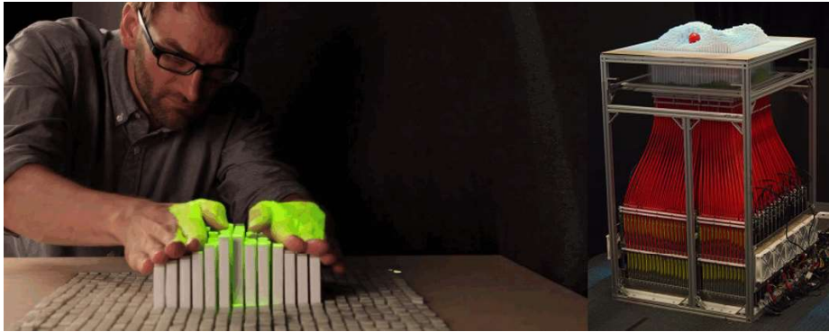
Fig. 2: MIT Media Lab's InForm system is a fully dynamic tangible display and interaction device with many applications. Courtesy Daniel Leithinger, Creative Commons License.
