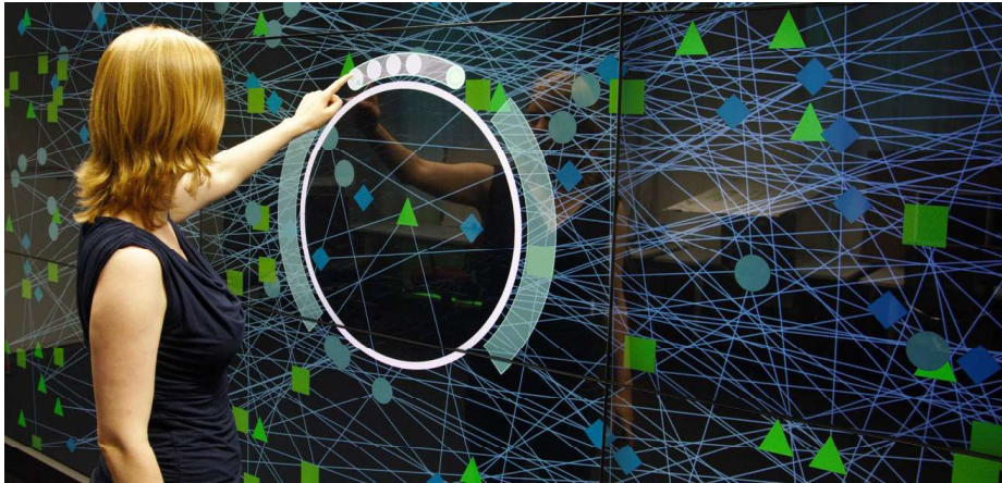
Fig. 9: A graph visualization using the BodyLenses system. The lens provides a personal embodied territory. The user can configure her lens with a touch menu.
